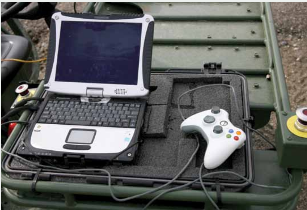
Marines use laptop computers to control robotic unmanned ground vehicles with payload capacity of 1,400 pounds that assist with transport requirements
